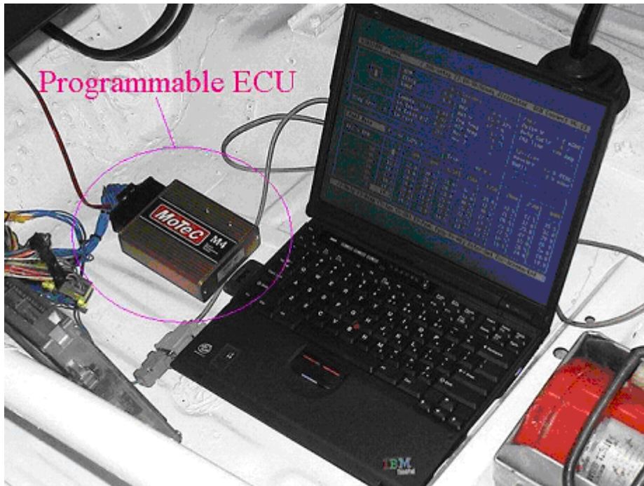
Fig. 2. Engine tune-up using programmable ECU
