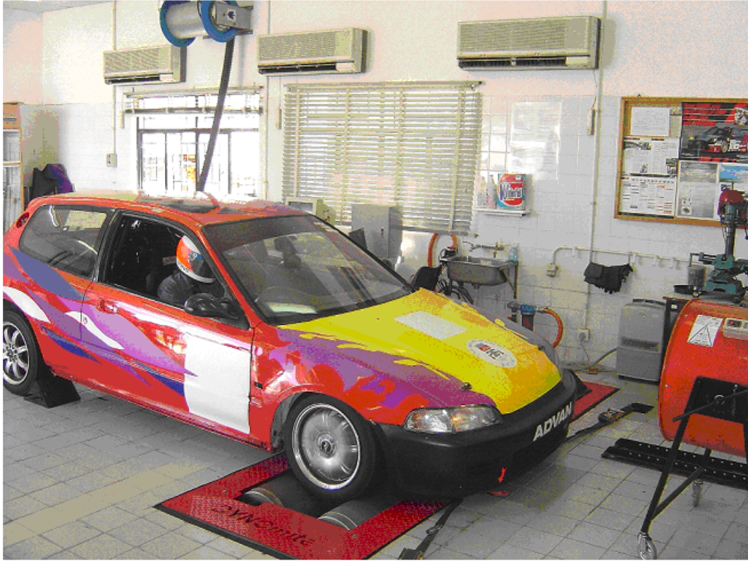
Fig. 7. Car engine performance data acquisition on a dynamometer
