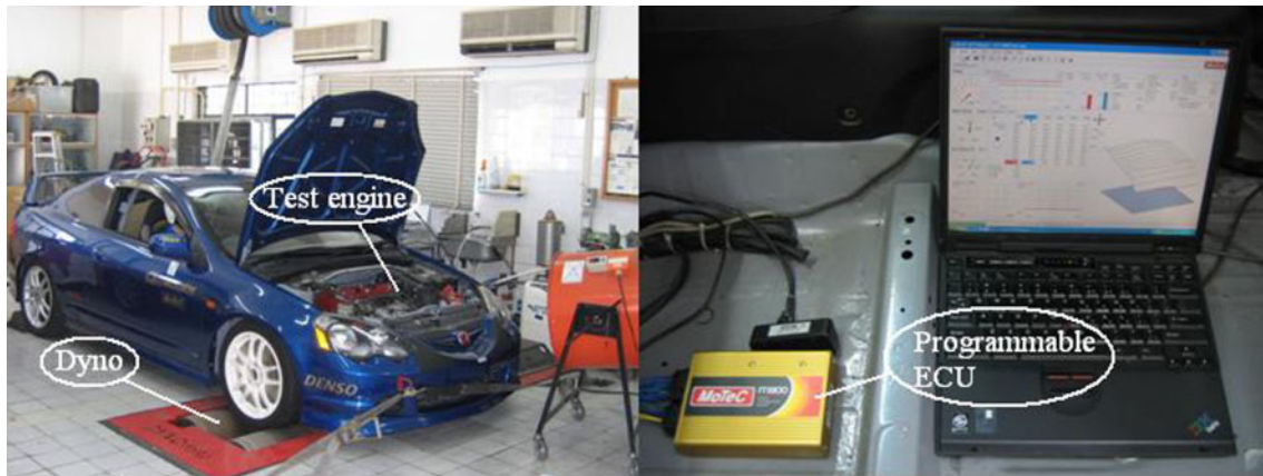
Fig. 3 Experimental set-up for data sampling and programmable ECU
